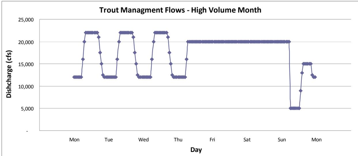
**Figure C-5.** Illustration of a Trout Management Flow experiment with a stranding flow in a high volume month. The stranding flow, as in a low volume months a 20,000 cfs constraint flow for three days, followed by a ramp down to 5,000 cfs.
