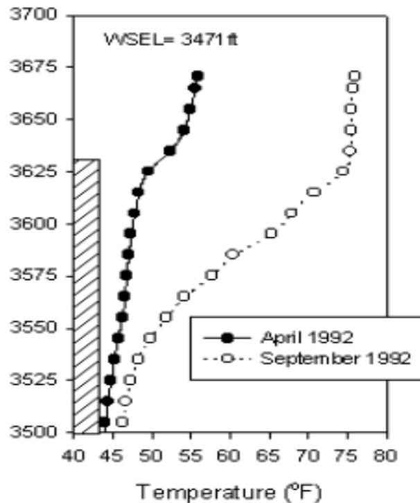
**Figure D-3.** Forebay temperature profiles for April and September 1992. Figure from Vermeyan (1999).
