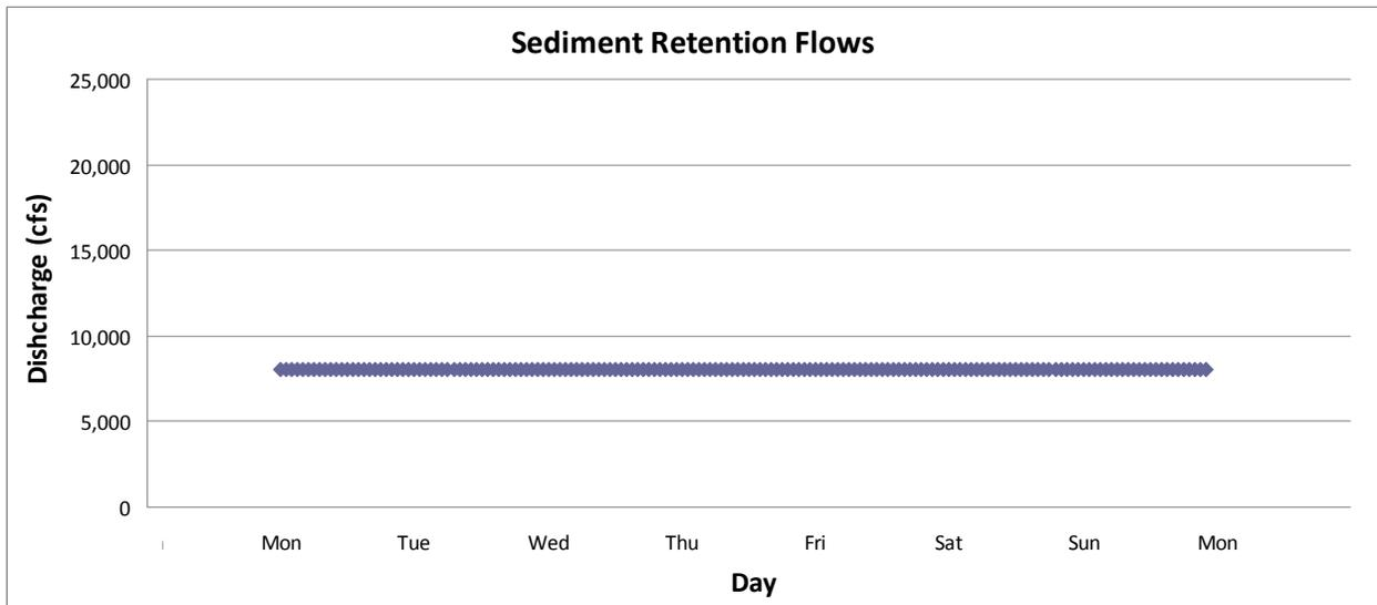
**Figure C-6.** Illustration of the “sediment retention flows” in a targeted monthly volume month. This would occur if there had been a significant, sediment-laden flow at the Paria River. The actual steady release may not be at exactly this magnitude of release. The release also wouldn’t be entirely without fluctuations due to operational changes, however load-following would be curtailed.
