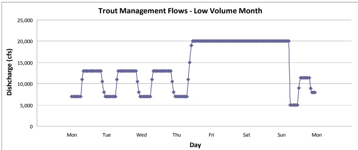
**Figure C-4.** Illustration of the concept a Trout Management Flow experiment. The one illustrated in this graph is a stranding flow experiment in a low volume month. The specifics of this experiment would need to be determined and tested. In this illustration, water release is brought up to 20,000 cfs for three days and then rapidly ramped down to 5,000 cfs. The intervening base flow regime is returned to between treatments.
