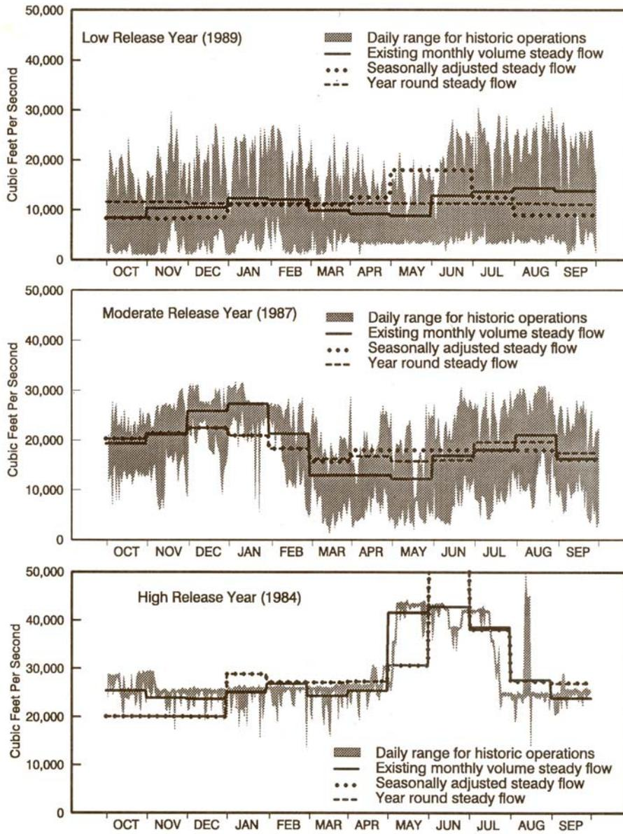
**Figure D-1.** Steady flows compared to No Action for low, moderate, and high release years. From 1995 EIS (Reclamation 1995).
