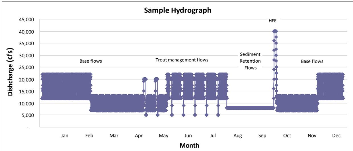
**Figure C-1.** Annual hydrograph illustrating a base flow that includes higher volume months, lower volume months, targeted monthly volumes (sediment conservation) in August through October, an HFE in November and Trout Management Flow experiments from May through July. This is an illustration of a year four of Table 2a. The remaining figures will illustrate the various components of this year.
