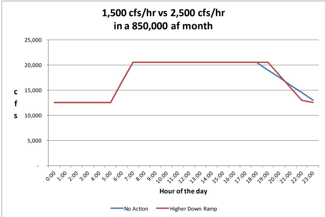
**Figure C-9.** Comparison of a 1,500 cfs/hr downramp rate with a 2,500 cfs/hr in a 850,000 af month.
