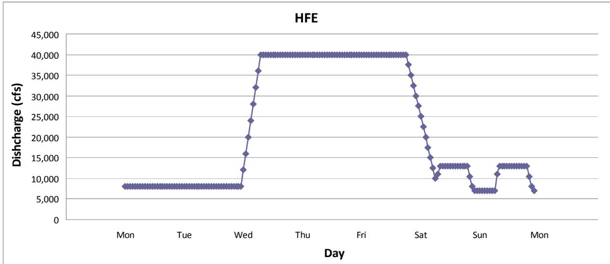
**Figure C-7.** A graphical illustration of an HFE. This particular HFE is 96 hours long during its peak. Operations preceding the HFE are depicted as sediment conservation flows and normal operations for a low volume month (October) begin at the conclusion of the HFE.
