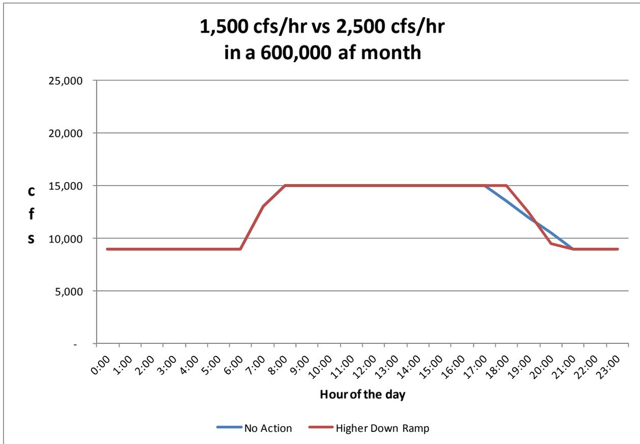
**Figure C-8.** Comparison of a 1,500 cfs/hr downramp rate with a 2,500 cfs/hr in a 600,000 af month.
