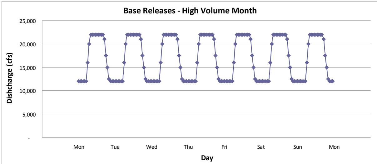
**Figure C-3.** Illustration of a week of a base flow in a higher volume month. These months are more likely in the peak power months of December, January, February, June, July and August. The daily pattern includes load following with a downramp rate of 2,500 cfs. The maximum daily change for load following is proportional to the monthly volume (in cfs).
