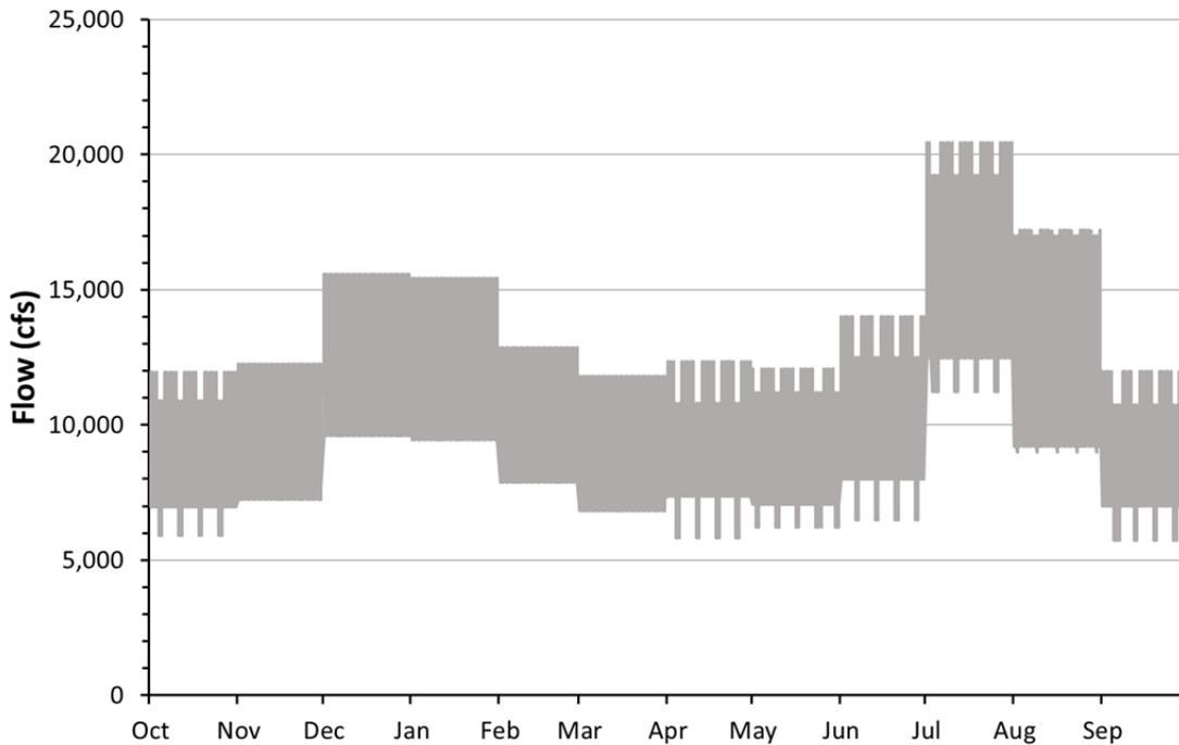
**FIGURE 2-2 Simulated Hourly Flows under Alternative A in an 8.23-maf Year (Note that there are differences in the mean, maximum, and minimum flows shown here and in Figure 2-1. These differences reflect flexibility in operational patterns allowed within the constraints of the alternative.)**
