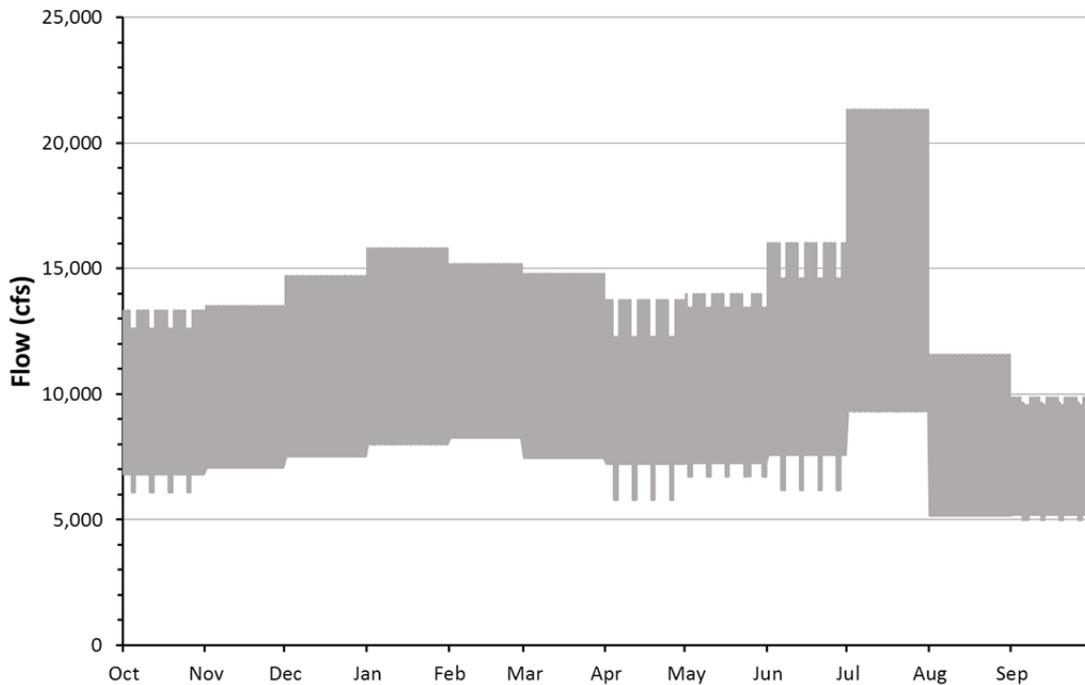
**FIGURE 2-24 Simulated Hourly Flows under Alternative E in an 8.23-maf Year (Note that there are differences in the mean, maximum, and minimum flows shown here and in Figure 2-23. These differences reflect flexibility in operational patterns allowed within the constraints of the alternative.)**
