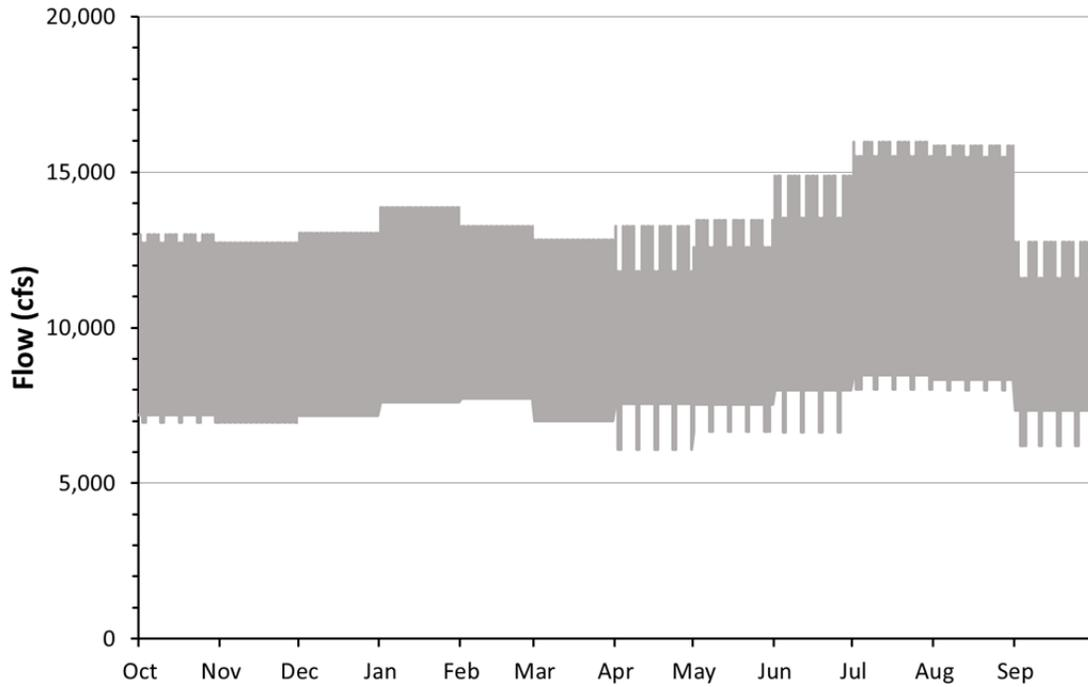
**FIGURE 2-18 Simulated Hourly Flows under Alternative D in an 8.23-maf Year (Note that there are differences in the mean, maximum, and minimum flows shown here and in Figure 2-17. These differences reflect flexibility in operational patterns allowed within the constraints of the alternative.)**
