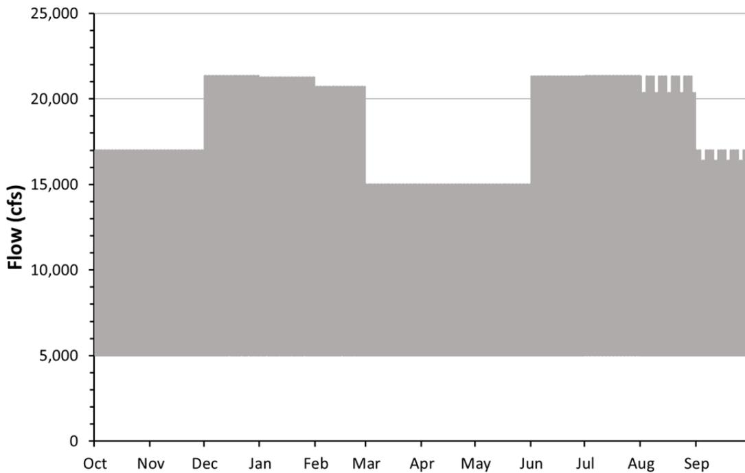
**FIGURE 2-8 Simulated Hourly Flows for a Hydropower Improvement Experiment under Alternative B in an 8.23-maf Year (Note that there are differences in the mean, maximum, and minimum flows shown here and in Figure 2-7. These differences reflect flexibility in operational patterns allowed within the constraints of the alternative.)**
