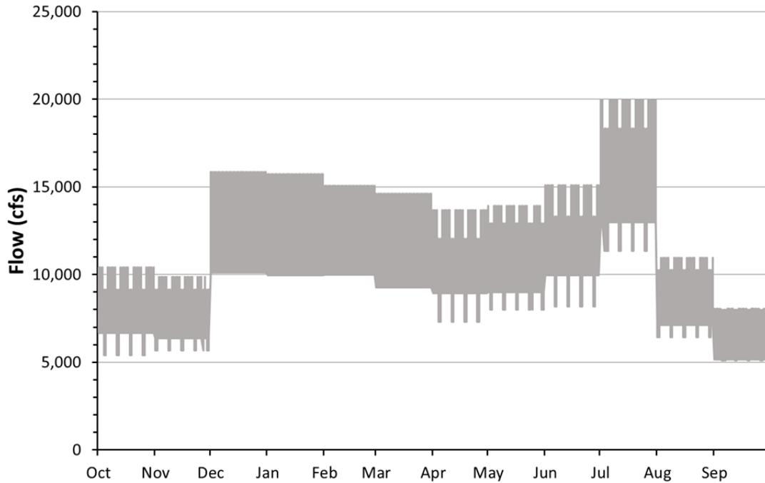
**FIGURE 2-11 Simulated Hourly Flows under Alternative C in an 8.23-maf Year (Note that there are differences in the mean, maximum, and minimum flows shown here and in Figure 2-10. These differences reflect flexibility in operational patterns allowed within the constraints of the alternative.)**
