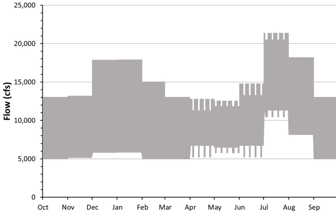
**FIGURE 2-5 Simulated Hourly Flows under Alternative B in an 8.23-maf Year (Note that there are differences in the mean, maximum, and minimum flows shown here and in Figure 2-4. These differences reflect flexibility in operational patterns allowed within the constraints of the alternative.)**
